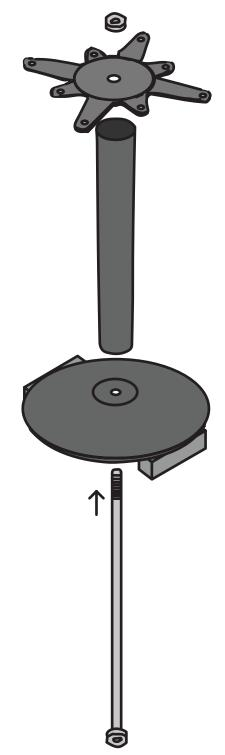
\*Note: If your assembly rod has removable nuts at both ends (instead of a welded square at one end), it can be used in either direction. Some Argent-28 models may have two assembly rods.
